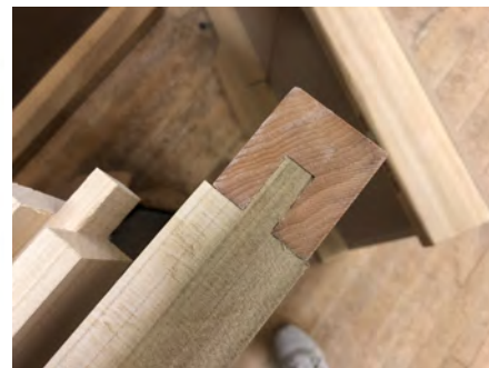
Figure 9: Drawings showing tenon and mortise joinery and picture of real joinery on the frame
