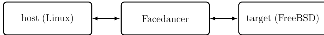
Figure 6.1: Diagram of testing setup. Software (in this case, umap) running on the “testing host” (left) causes the Facedancer to emulate a variety of USB devices when connected to the “target” (right).
