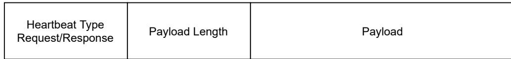
Figure 3.1: Syntax of a Heartbeat message in TLS. The client sends a request and expects to receive an identical response with just the packet type changed.
