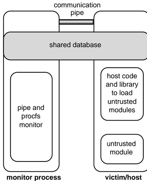
The “new untrusted module” message is sent to the `monitor` when a new module has been loaded into memory and placed in the database. Included in this message is the address of the `EscapeTable`. Next, the `monitor` writes the callback addresses into the table.
