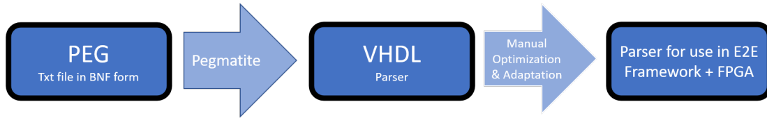
Figure 1.1: Process for generating optimized parsers
