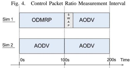
**Metric 2:** Ratio of unicast and multicast control packets per data packet sent from UDP layer i.e., *the control packet ratio*. This metric helps us evaluate the efficiency of the destination protocol after swap.
