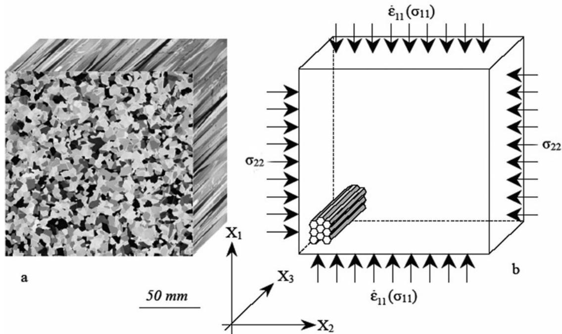
**Fig. 1.** (a) Composite polarized photograph of laboratory-grown freshwater ice specimen microstructure. (b) Schematic representation of loading stage. In the proportional-loading procedure  $\sigma_{22} = R\sigma_{11}$ . In the constant minor stress procedure  $\sigma_{22}$  is constant.
