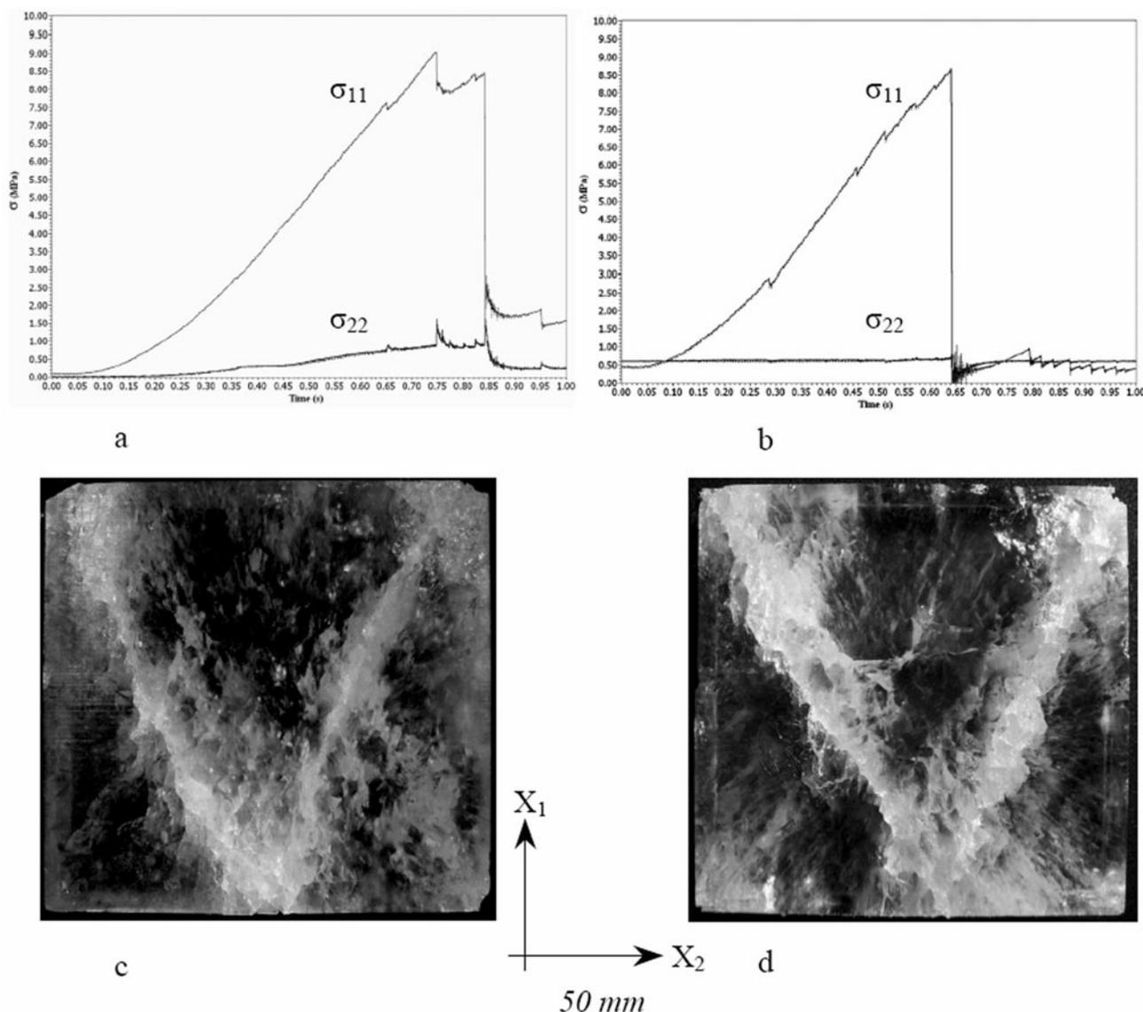
**Fig. 3.** (a, b) Stress–time curves from (a) a proportionally loaded test and (b) a constant minor stress test. (c, d) Photographs of a faulted specimen ( $X_3 = \sim 50$  mm) showing conjugate faults from (c) a test performed under proportional loading, corresponding to the stress–time curve in (a), and (d) a test performed under constant minor stress, corresponding to the stress–time curve in (b).
