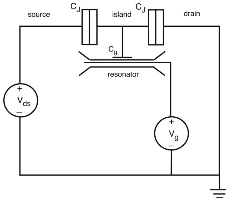
**Figure 1.** Model circuit of the SSET-resonator system.
