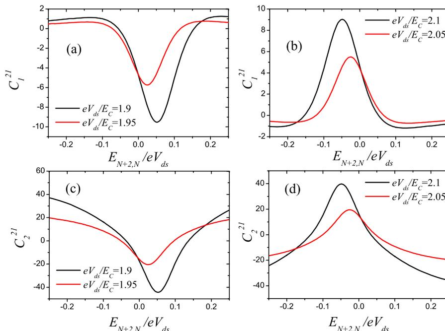
**Figure 6.** Numerical calculations of the coefficients  $C_1^{21}$  and  $C_2^{21}$  in the vicinity of the DJQP resonance. The different values of  $E_C/eV_{ds}$  correspond to points at different distances below, (a) and (c), and above, (b) and (d), the centre of the DJQP resonance (see figure 5). As before, we choose  $\epsilon_J = 1/16$ ,  $r = 1$  and set the quasi-particle tunnel rates and their gradients to unity.
