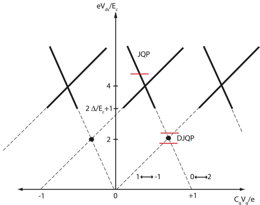
**Figure 5.** Schematic map showing the location of a selection of neighbouring JQP resonances (solid black lines) and DJQP resonances (solid black circles). The bias ranges for the  $C_1^{21}$ ,  $C_2^{21}$  and  $T_{\text{SET}}$  plots are indicated by the solid red lines.
