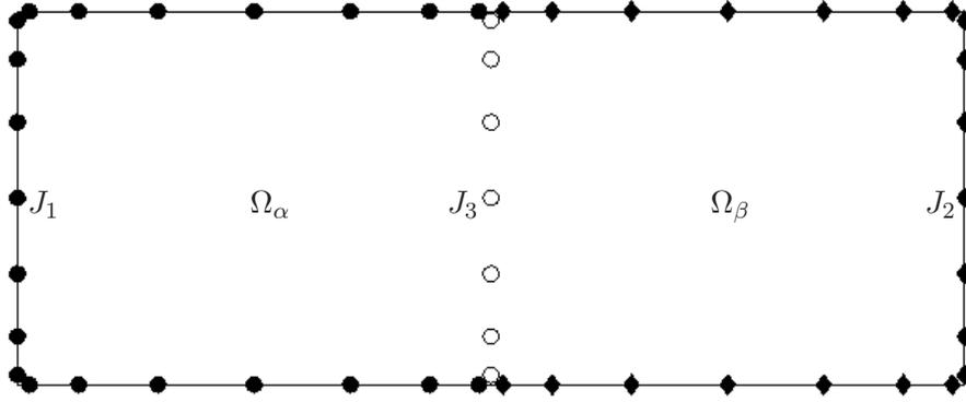
FIGURE 3. Notation for the merge operation described in Section 4. The rectangular domain  $\Omega$  is formed by two squares  $\Omega_\alpha$  and  $\Omega_\beta$ . The sets  $J_1$  and  $J_2$  form the exterior nodes (black), while  $J_3$  consists of the interior nodes (white).
