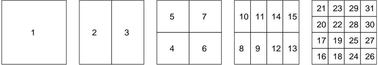
FIGURE 1. The square domain  $\Omega$  is split into  $4 \times 4$  leaf boxes. These are then gathered into a binary tree of successively larger boxes as described in Section 5.1. One possible enumeration of the boxes in the tree is shown, but note that the only restriction is that if box  $\tau$  is the parent of box  $\sigma$ , then  $\tau < \sigma$ .
