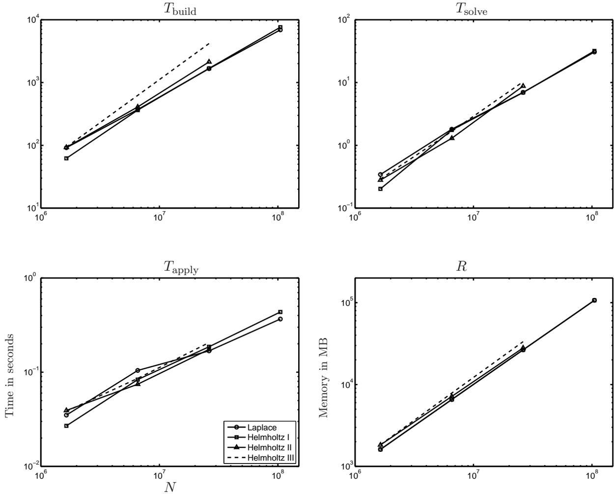
FIGURE 6. The first three graphs give the times required for building the direct solver ( $T_{\text{build}}$ ), solving a problem ( $T_{\text{solve}}$ ) and applying the approximate Dirichlet-to-Neumann operator on  $\partial\Omega$  ( $T_{\text{apply}}$ ). The fourth graph gives the memory  $R$  in MB required to store the solution operator.
