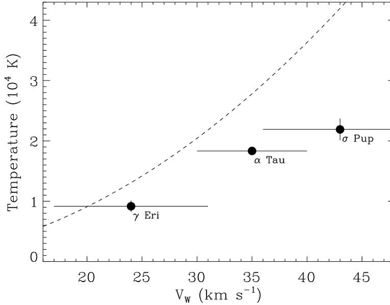
**Figure 5.** The post-TS temperature estimated from the astrospheric Mg II lines in Table 2 is plotted versus the stellar wind velocity estimates from Table 1. The dashed line is the relation expected for a simple hydrodynamic shock at the strong shock limit, assuming a pure hydrogen fluid.
