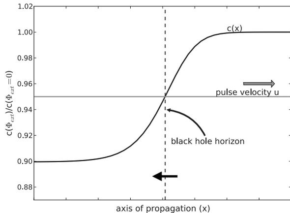
FIG. 2: Effect of a step-like flux pulse on the propagation velocity of a JJA as seen in the comoving frame. The pulse velocity was chosen to be  $u = 0.95c(\Phi_{\text{ext}} = 0)$ . The black hole horizon occurs where  $c(x) = u$ . Arrow indicates the only permissible direction of travel across the horizon.
