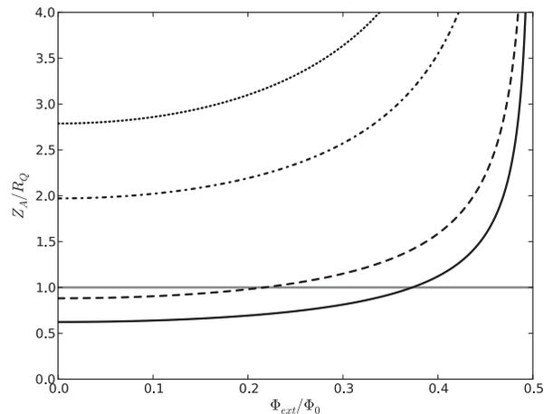
FIG. 3: Ratio of array impedance  $Z_A$  to the resistance quantum  $R_Q$  as a function of the external flux bias for a critical current  $I_c = 2\mu\text{A}$  and example ground capacitor values:  $C_0 = 10^{-16}$  (solid),  $5 \times 10^{-17}$  (dashed),  $10^{-17}$  (dash-dot), and  $5 \times 10^{-18}$  F (dotted). High and low impedance regions are defined above and below  $Z_A/R_Q = 1$  respectively.
