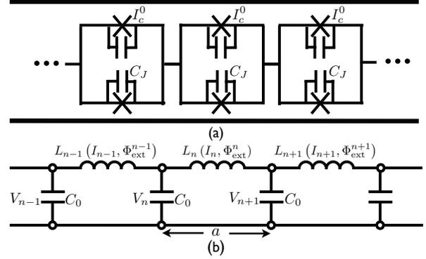
FIG. 1: a) Layout of the dc-SQUID transmission line. We assume each SQUID element is formed from identical tunnel junctions with critical current  $I_c$  and capacitance  $C_J$ . b) Effective lumped circuit model valid for frequencies below the plasma frequency and negligible SQUID self-inductance.
