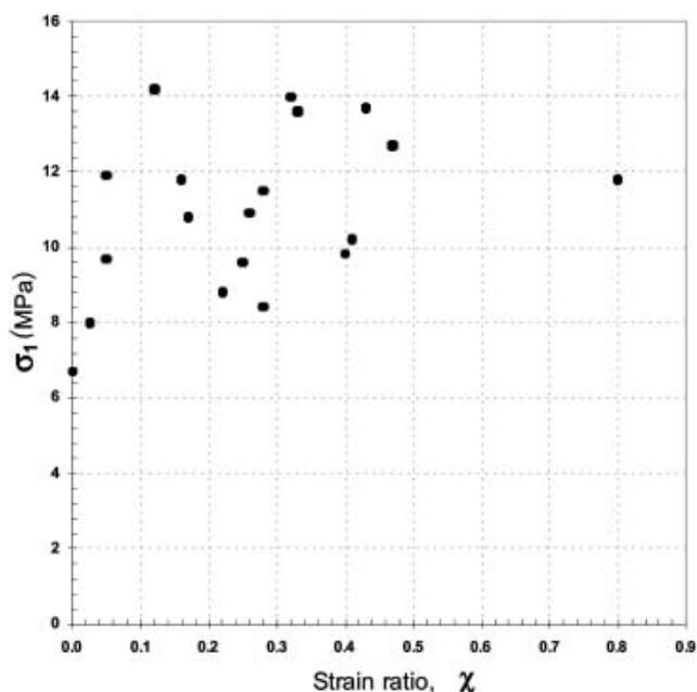
**Fig. 1.** Graph of terminal failure stress vs applied strain ratio for S2 columnar-grained fresh-water ice of  $6 \pm 2$  mm column diameter deformed through proportional straining across the columns at  $-10^\circ\text{C}$  at a strain rate (along the direction of shortening) of  $4.5 \pm 1.5 \text{ s}^{-1}$ .
