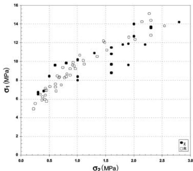
**Fig. 2.** Graph of terminal failure stress vs confining stress for the material described in Figure 1, showing data obtained through proportional straining tests ( $\chi$ ; closed symbols) and data obtained by Iliescu and Schulson (2004) through proportional loading ( $R$ ; open symbols). (Note that Figure 1 contains four fewer points than this figure because lateral strains were not recorded in four tests.)
