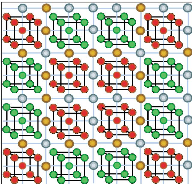
FIG. 2 (color). Magnetization patterns with cubic symmetry for  $\text{Fe}_9\text{Al}_7$  with the magnetic unit cell doubled in each direction to form a structure that would produce magnetic scattering related to that observed in Fe(43Al). The first three layers of the 1024-atom unit cell are shown with the coding of Fig. 1.
