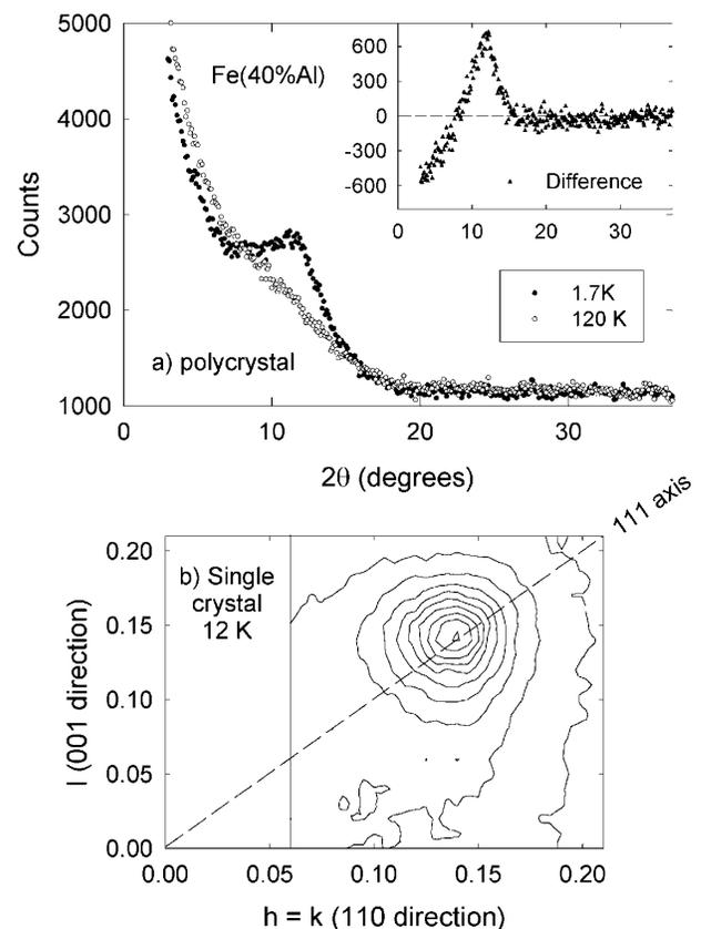
FIG. 3. Neutron scattering intensity for (a) polycrystalline Fe(40Al) at 120 and 1.7 K with their difference shown in the inset and (b) single crystal Fe(40Al) at 12 K shown as contours about the  $(\frac{1}{7}, \frac{1}{7}, \frac{1}{7})$  peak.
