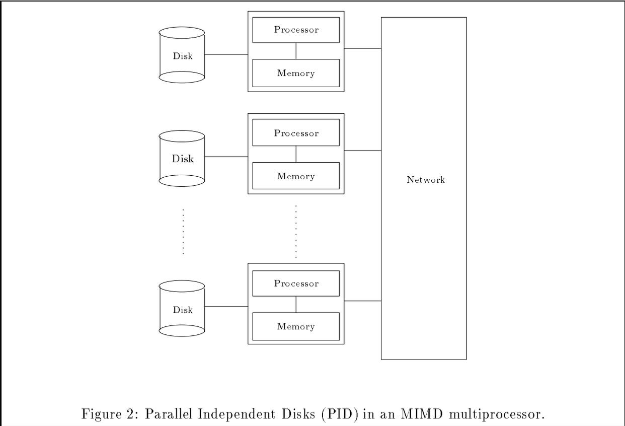
Figure 2: Parallel Independent Disks (PID) in an MIMD multiprocessor.
