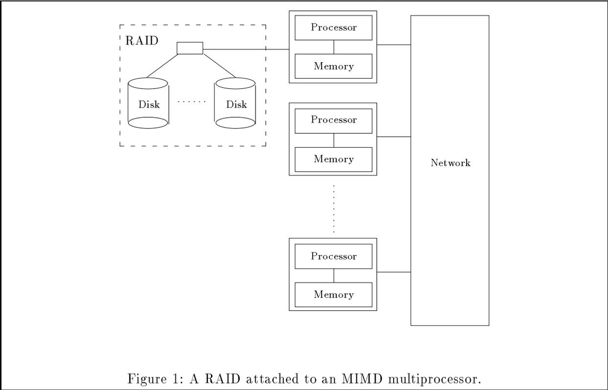
Figure 1: A RAID attached to an MIMD multiprocessor.
