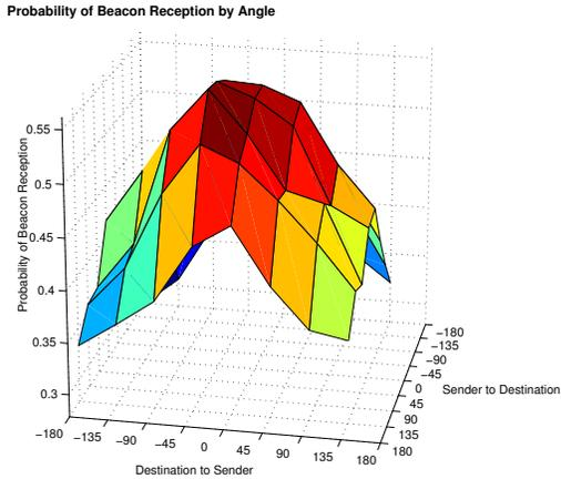
**Figure 1:** The probability of beacon reception as a function of the two angles, the angle between the sender’s antenna orientation and the receiver’s location, and the angle between the receiver’s antenna orientation and the sender’s location. In this plot, we divide the angles into buckets of 45 degrees each.
