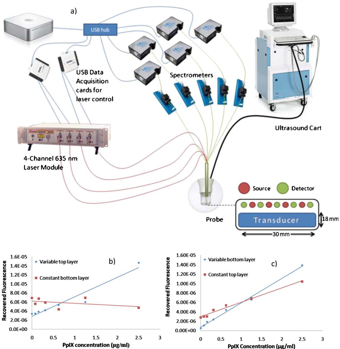
**Fig. 1** The system schematic is illustrated in (a) showing components and probe geometry, with data acquisition from five compact spectrometers. The recovered fluorescence values for the layers (b) with the top concentration varied and the bottom fixed at  $0.625 \mu\text{g/ml}$ . In (c), the top layer was held constant and the bottom layer varied.
