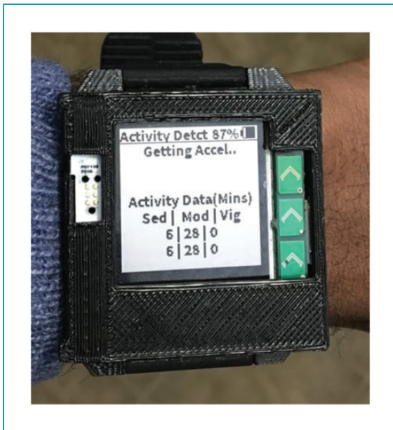
Figure 2. This application evaluates the activity of an individual and classifies it as low, moderate or vigorous.
