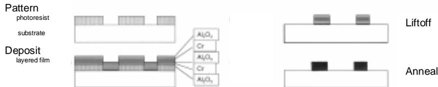
Fig. 2 Sample preparation process
