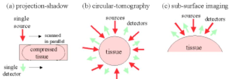
**Fig. 1.** Schematic of three typical source-detector geometries used in diffuse optical tomography applications. The projection-shadow geometry (a) is used in several optical mammography scanners [3, 23-25], while the circular-tomography geometry (b) is used for both breast and brain imaging [16, 26], as is the sub-surface imaging geometry (c) [2, 27, 28].
